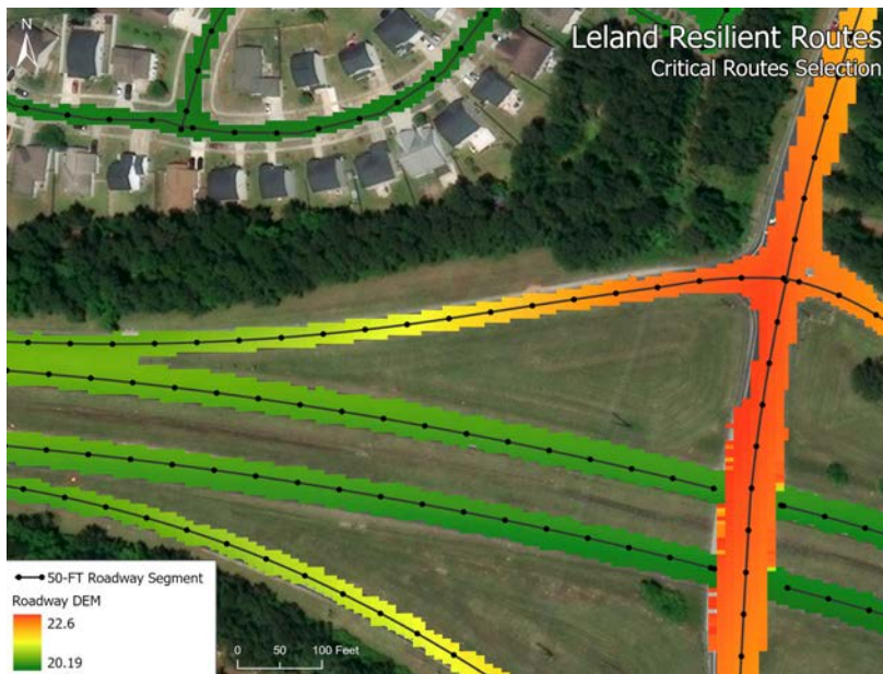
Figure 3: Routes split into 50-FT segments overlying a terrain DEM
